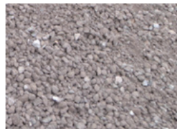
Gravel after recycling
